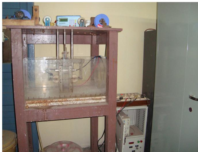
Figure 3: TW-ECDM System Set up
